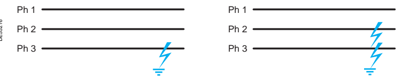
Fig. 3. Phase-to-earth short-circuit (80% of cases).
