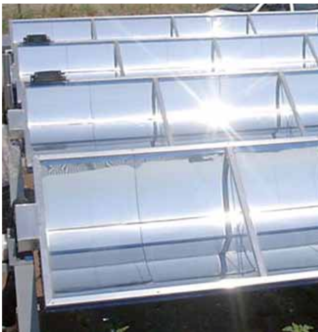
Figure B.5 – Parabolic trough concentrators
