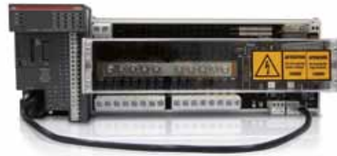
Substation PLC - AC500 series* Dimensions: 590 x 700 x 260
